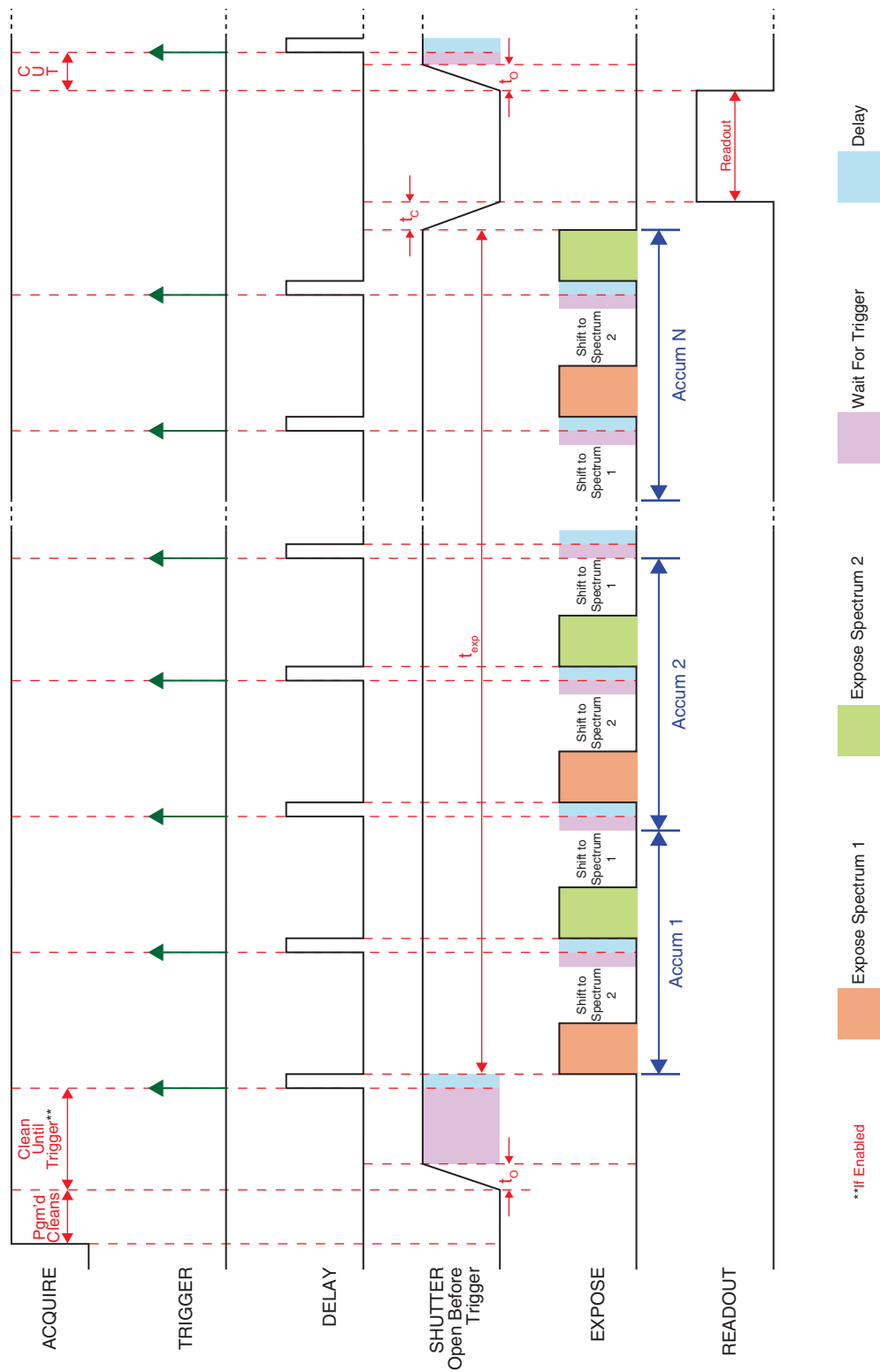
Figure 11-20:SeNsR Timing Diagram: Shift Per Trigger, Open Before Trigger
