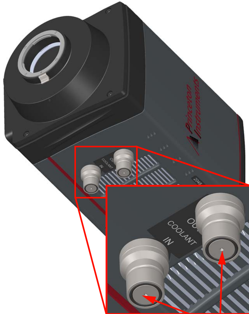
Figure D-2: Depressing Coolant Fittings' Center Pistons
