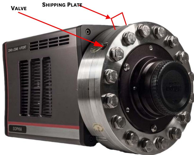
Figure E-1: Shipping Plate Mounted to Camera
