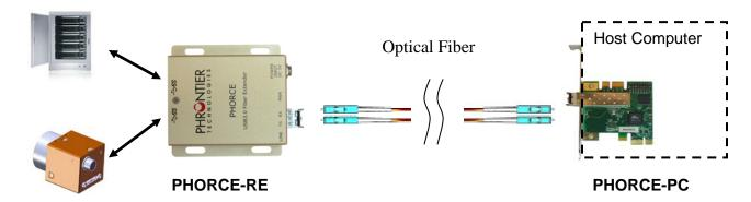
**Note:** Operation requires certain power-up sequence. The RE side must be powered on before the PC side while the optical link is connected. If the optical link is interrupted during operation, after the optical link is re-connected the system needs to be re-started with the correct power-up sequence.
