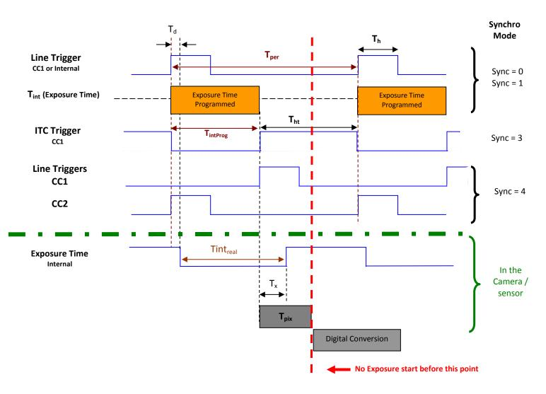
$\mathbf{T}_{pix}$ : Timing Pixel. During this uncompressible period, the pixel and its black reference are read out to the Digital converter. During the first half of this timing pixel (read out of the black reference), we can consider that the exposure is still active.
