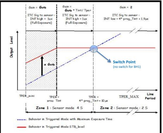
When the User selects a synchronization mode which requires the control of the exposure, the camera enters a specific mode:
