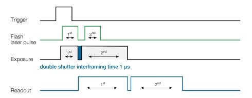
The duration of the first exposure time can be configured. The duration of the second exposure time is fixed and pre-defined by the readout time of the first image. Therefore, it is usually necessary to prevent the sensor from ambient light during the prolonged second exposure time.
