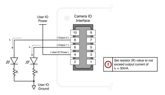
• Alternatively, one external LED can be connected in the Common Anode configuration.
