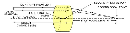
Figure 1: Primary Points in a Lens System
