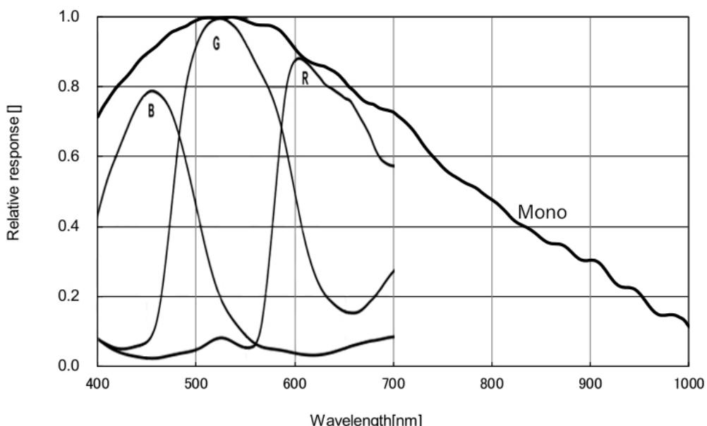
图 4-16 MER2-1220-32U3M/C(-L/-W90/-W90-S90) SENSOR 响应曲线
