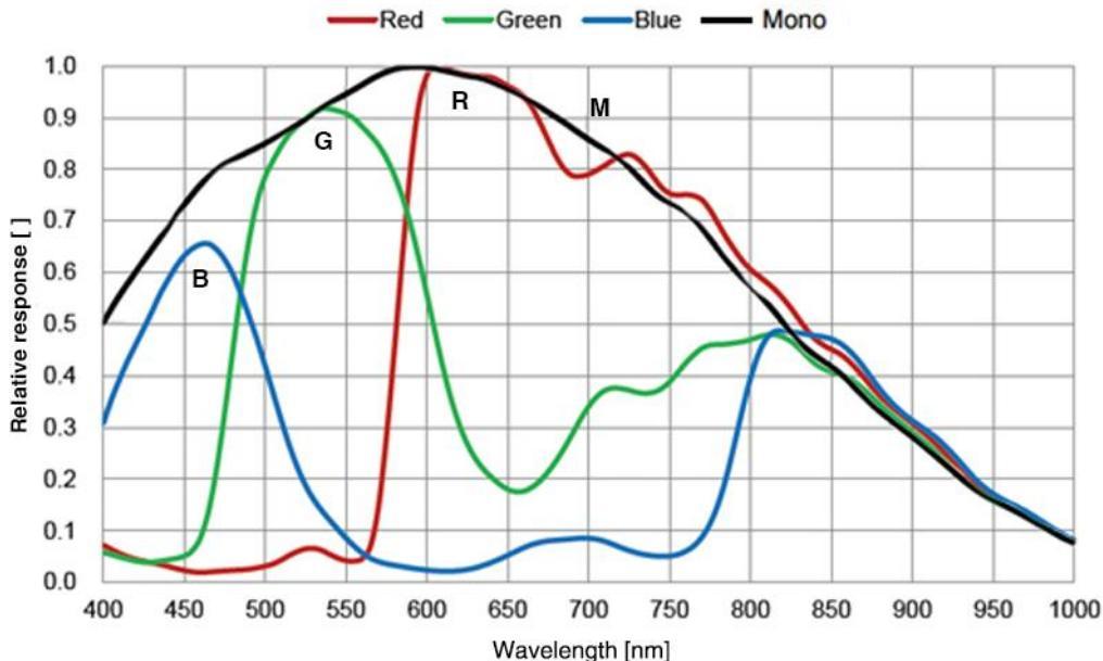
图 4-40 ME2L-161-61U3M/C(-L) SENSOR 响应曲线
