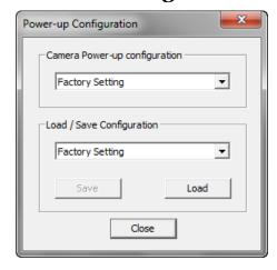
CamExpert provides a dialog box which combines the features to select the camera power up state and for the user to save or load a camera state from Linea CL memory.
