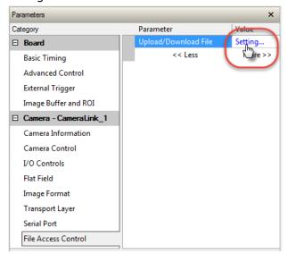
• From the file type drop menu, select the file type that will be uploaded to the Linea CL. This CamExpert tool allows quick firmware changes or updates.
