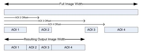
For example, in the 4k camera model, if the total number of pixels for the specified AOI`s is less than 1 K when using base Camera Link mode at 77 MHz, the maximum line rate can be 80 kHz; versus 56 kHz if all 4k pixels were output.
