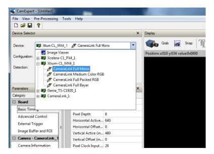
8. Modify the camera and frame grabber parameter settings as required. At present, when using GenCP cameras, the camera and frame grabber parameters must be adjusted separately. Test the image acquisition by clicking the **Grab** button.
