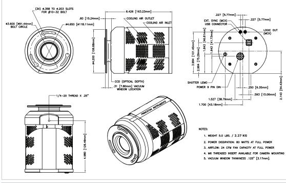
PIXIS with Spectroscopy Mount; with Shutter
