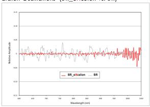
BR\_eXcelon eliminates much of the residual etaloning observed in the standard back-illuminated deep depletion ("BR") version.
