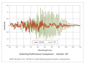
B\_eXcelon provides significantly lower etaloning (unwanted fringes) compared to standard back illuminated ("B") version.
