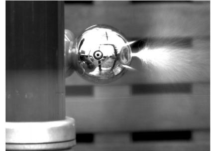
Corona discharge in air at the terminal of a transformer at 163 kV. With friendly permission of: Laboratory of High Voltage Engineering and Switchgear Technology, Technische Universität München, Munich, Germany [www.hsa.ei.tum.de](http://www.hsa.ei.tum.de)
