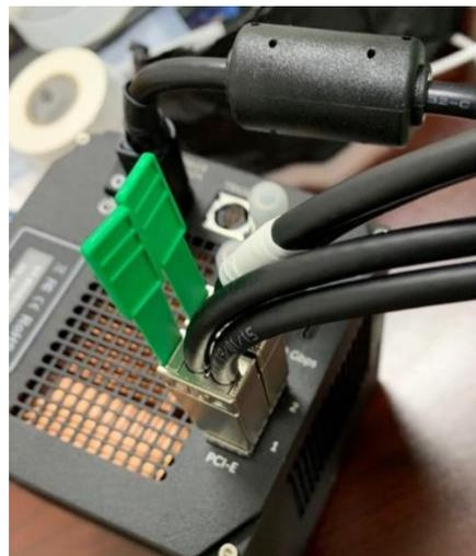
*PCIe cables inserted into camera's PCIe ports.*
