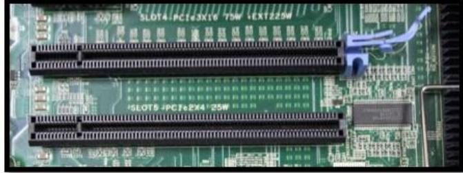
5. Hold the PCIe card (being careful not to touch the board components or PCIe bridge pins) and insert it, properly orientated, into the open slot. The card should slide into place with minimal resistance and click when fully inserted.
