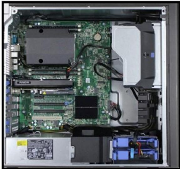
4. Locate an available 8-channel or higher PCIe slot (marked x8). Refer to the PC's documentation to locate a suitable slot.
