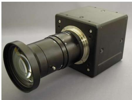
BV-C3350 uses a beam splitter and two line sensors which each sensor has different focal points. Therefore, BV-C3350 can get two images with the different focal points at the same time and with the same field of view. This function will be convenient for a glass cover investigation on surface and inside, for instance. As BV-C3350 sets the sensor position based on customer applications, this is a custom-made product.
