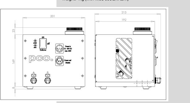
All dimensions are in millimeters. Weight: 4kg (with filled coolant tank)
